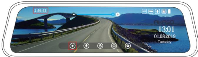
The time displayed in the top-left corner indicates how much time is left for the inserted card to record. After recording some videos, the time will be reduced accordingly; when the time display "0:00:00", that means the card is full. If turning on "Loop Record", you don't need to change or format the card, it still records and the newest file will automatically overwrite the oldest file.
